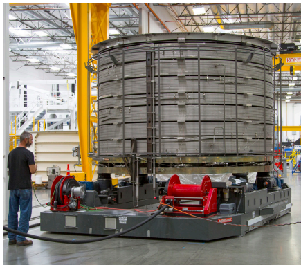
First module on air transporter moving to heat treatment furnace
